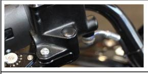
Remove the original mirrors and push the plastic coverings provided into the thread.
