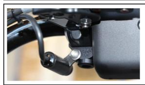
*Tip: The screw and washer provided can be used to attach the switch of an adjustable exhaust system to the clamp.*
