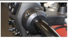
Remove the two original clamps and attach the mirror clamps using the original screws.
