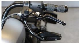
Attach the mirrors (using M10x1.25) to the clamps.
